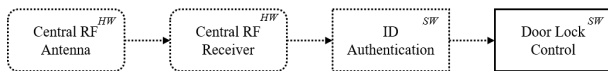
Fig. 16. The functional analysis architecture for the RKA fragment in the door locks system
