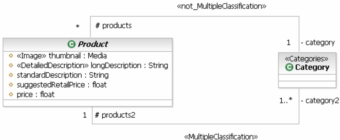
Figure 7.3: Using Multiple Associations to Model Multiplicity Variability 45
